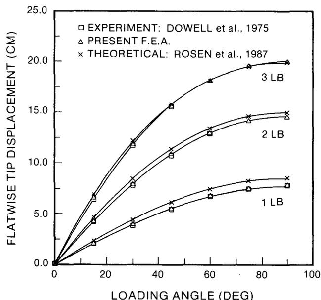
Fig. 2(b) Flatwise tip displacement
