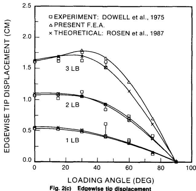
Fig. 2(c) Edgewise tip displacement
